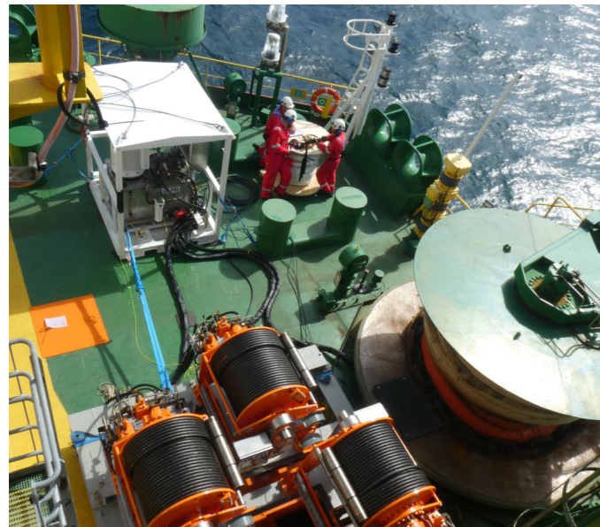
(Photo: Alpa Winch used in a thruster replacement project)
